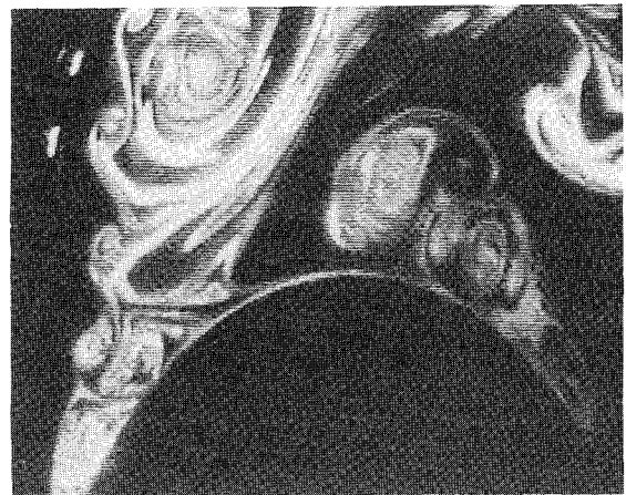
Fig. 3 Sample photograph displaying the effect of freestream secondary flows on the geometry of the stream surfaces in the lee of a 3.5 l/D ogive, with a sharp tip ( \alpha = 45 deg, x/D = 2.0 , and Re_D = 7.9 \times 10^3 ).
